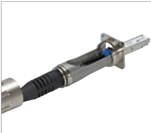
Remove LC dust caps and plug LC duplex connectors into SFP module
