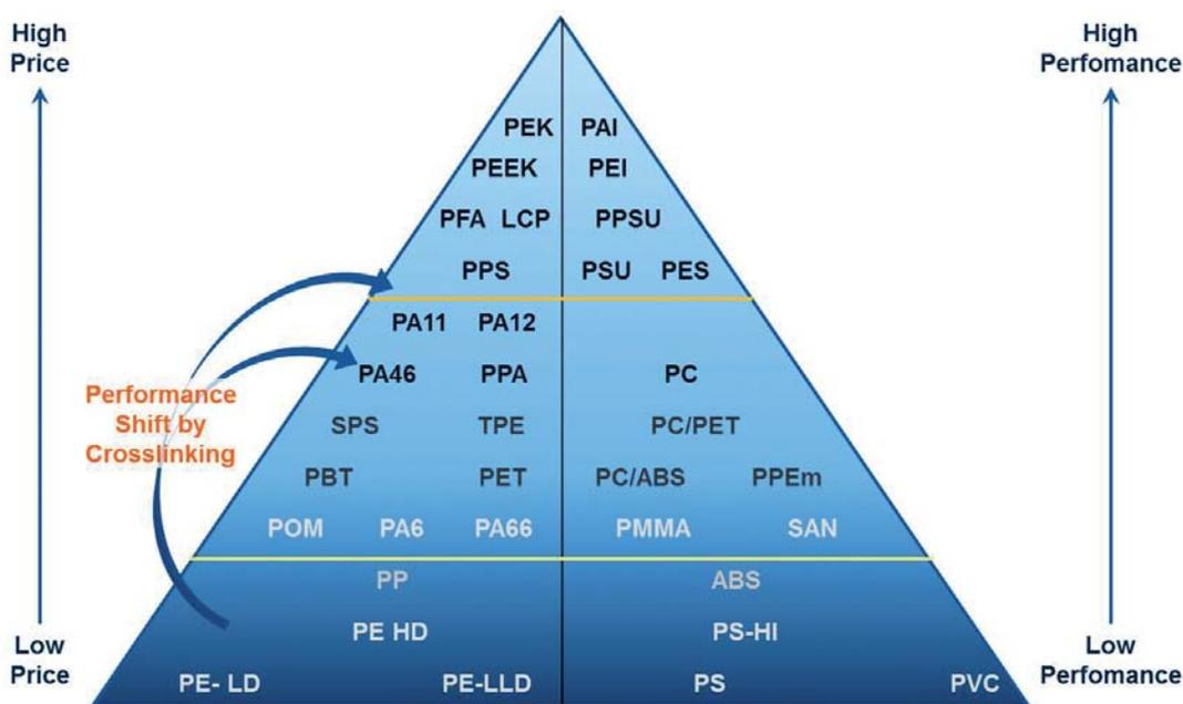
Figure 1: Improvement of material performance by crosslinking
